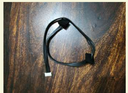
SATA COMMUNICATION CABLES
